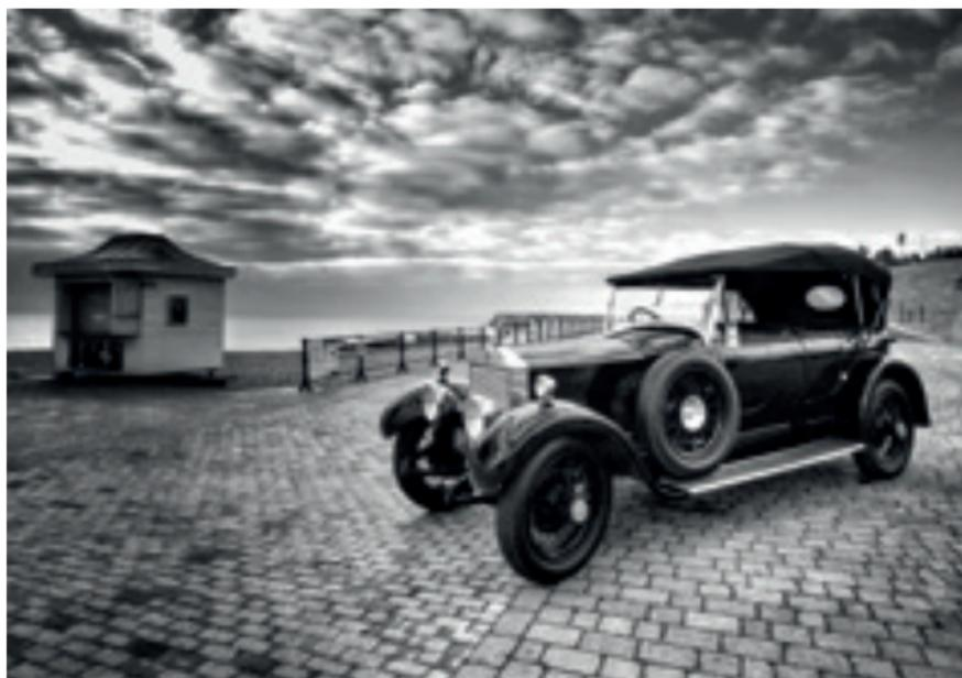
This particular car was built at The Rolls-Royce works in Nightingale Road, Derby and first road tested in 1927. Like all Rolls-Royce motor cars (prior to 1946) it was supplied as a rolling chassis. This particular chassis was pre-ordered by Barker & Co Ltd, coachbuilders (a London company founded in 1710 and who bodied the world's most valuable car – a Rolls-Royce Silver Ghost valued at \$57 million).
